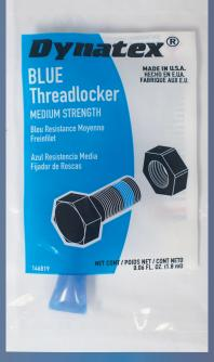
Dynatex Blue Medium Strength Threadlocker is designed for locking threaded fasteners that require disassembly with standard hand tools. The product performs on aluminum, steel, plated parts, stainless steel, and special alloy parts. Dynatex Blue Medium Strength Threadlocker exhibits good temperature and is solvent resistant.
